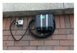
Photo 9.1: Typical Vibrograph installation
