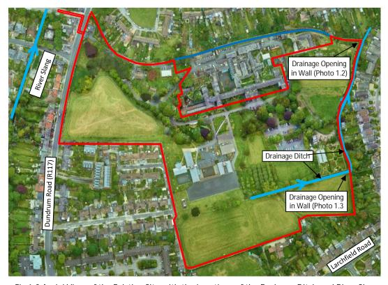
Fig 1.2 Aerial View of the Existing Site with the Locations of the Drainage Ditch and River Slang
